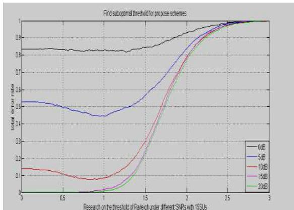
Fig. 3. Relationship between the total error probability and the threshold in the listening channel when the SNR in the reporting channel is 25 dB, and the listening channel has a different SNR.
